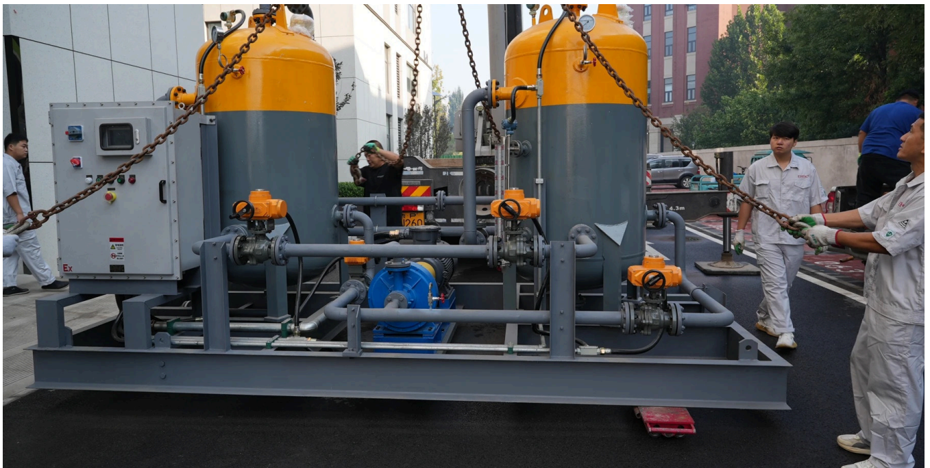
Complete pump skid being loaded for delivery.
