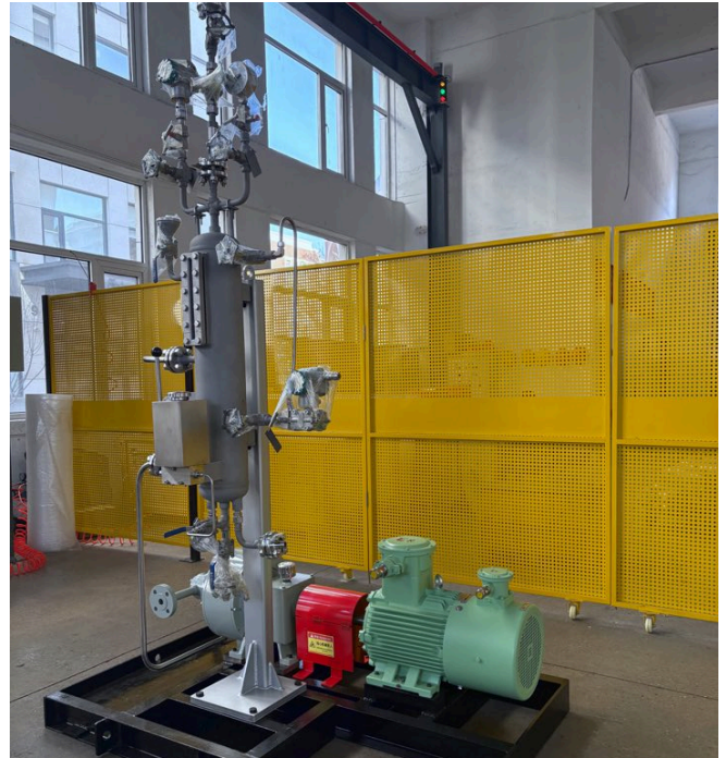
Pump set with a seal support and flush system
